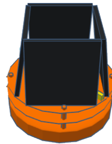
(b) Antenna configuration rotated 45^\circ with respect the initial design, placed at around 30cm from the ground, named Diamond.
