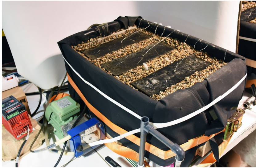
Figure 3.1.2 Photograph of one of the CW-MFC+ systems
