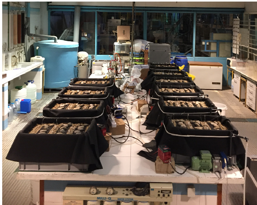
Figure 3.1.3 Photograph of the experimental setup with the eight experimental CW-BES (two additional test systems are in the right back)
