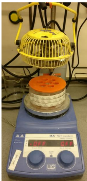
Figure 4.31: Photoreactor used for the reactions of aliphatic acyl chlorides.
