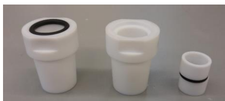
Figure 4.29: Teflon adaptors to use Schlenk tubes in the photoreactor.
