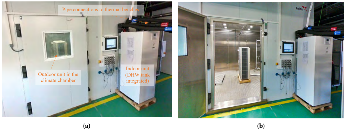
Figure III.4. Photograph of the laboratory with the floor standing indoor unit of the heat pump, and the outdoor unit in the climate chamber which is closed in (a) and open in (b).
