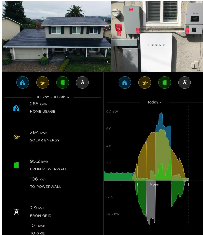
Fig. 1.1: Household load profile with photovoltaic power generation, storage and electric vehicle under an energy management system from Tesla, Inc. Courtesy of [24]
