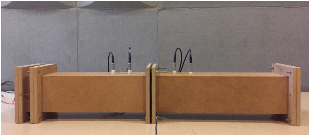
FIG. 16 Experiment setup for normal-incidence transmission loss measurements. (a) Schematic representation showcasing the four microphone positions and holding of the sample panel. (b) Actual impedance tube employed in the experiments. Figure from Article III.
