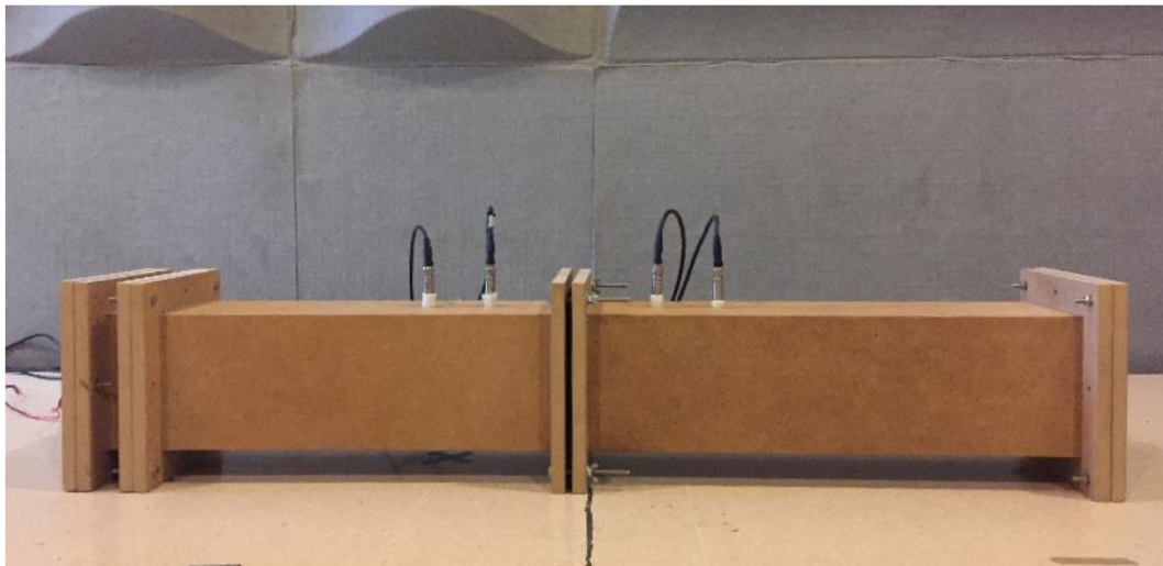
FIG. 1 Experiment setup representation of the impedance tubes used for measuring the normal incidence sound transmission loss of a sample LRAM panel. The tube cavity has a 8 cm \times 8 cm squared section and each pair of microphones are separated 7.6 cm apart. The frequency range of operation goes from 500 to 2000 Hz. All measures in the figure represent cm. (a) Schematic representation and (b) actual experimental setup.
