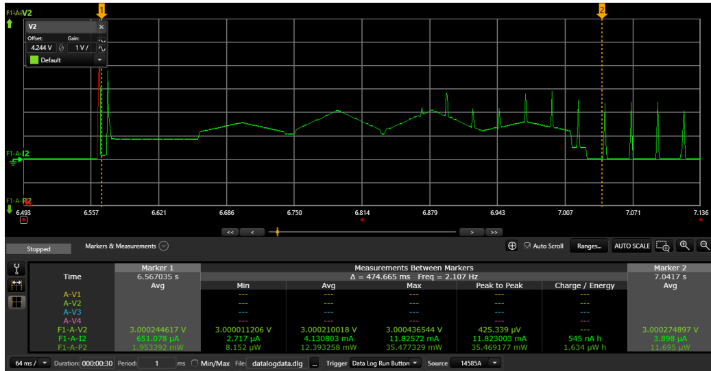
Figure 44: Current consumption pattern of the 6LBR during initialization
