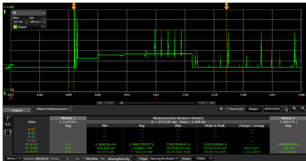
Figure 37: Current consumption of a 6LN during initialization
