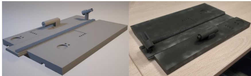
Figure 3: Elaboration of a lab scale sprayer model. Starting with the image located at the top, a basic concept of a laboratory sprayer is depicted. At the upper part of the core structure, a small motor rotates the stents while a resistance is used to control the rotation speed. At the bottom, another motor rotates with a gear attached to its end which is used to slide the sprayer's nozzle side-ways following the direction shown by the yellow arrow. Under this first image, a dimetric view of the core structure shows indentations made to place the motors, circular indentations for the resistances and perforations used to pass all the cables under the surface. A tray is designed to slide on one axis through a step design which prevents all other movements. Mounted on the tray, a holder is designed to fix the sprayer's nozzle. On a semicircular mount, a cylindrical piece is placed to enable the transmission of the rotation from the motor to a different type of outlet used to hold the stents. A last image located at the bottom shows a 3D model printed and ready to be customized.
