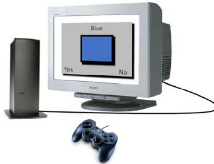
Figure 2.13 – Setup for our psychophysical experiment. Color patches and color names were presented on a calibrated CRT monitor and the observer pressed buttons on a gamepad to decide whether the color patch was well described by the name or not. The background was mid-grey and a reference white was provided by a D65-colored frame.
