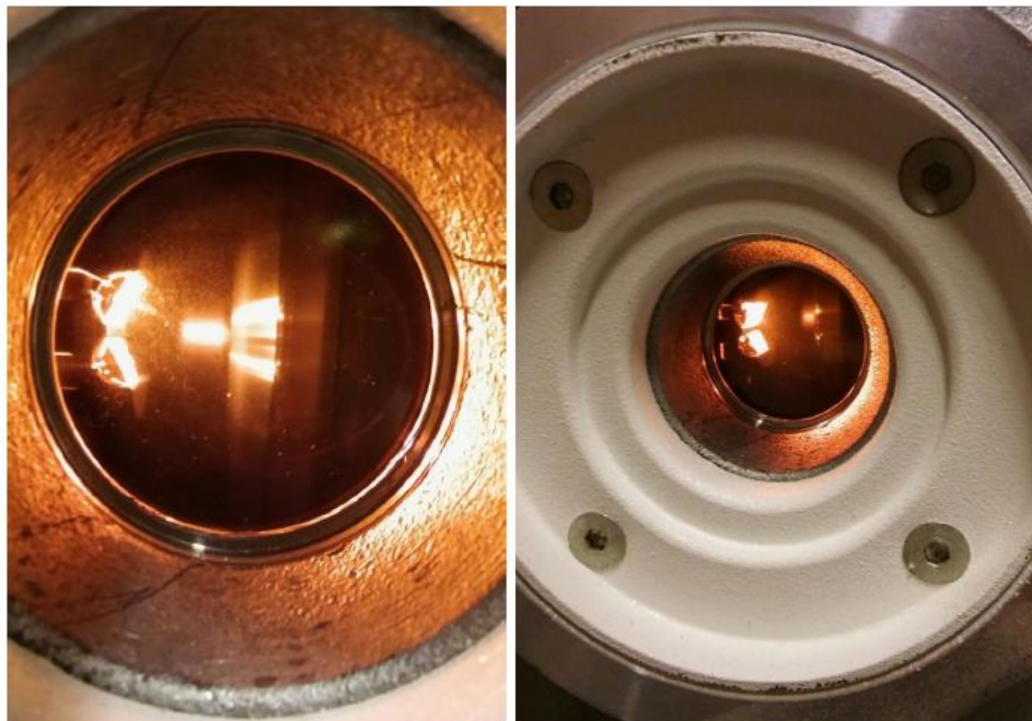
Figure 3.12 - X-ray tube filaments and optical projection on the anode. (Compare the cathode assembly to the scheme in Figure 1.4).
