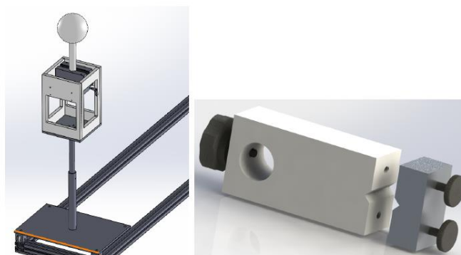
Figure 3.7 - Trolley and supports projects for a slim stem ionization chamber. The left image shows the support mounting along the mechanical bench while the right one shows the detail of a holder indent for positioning the detector stem.
