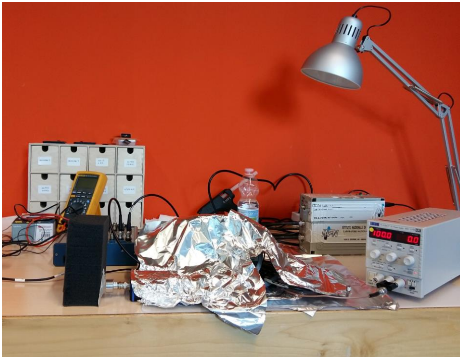
Figure 8.14 - CdTe calibration setup. The figure shows, from the left to the right, the positioning of the radioactive source, the CdTe detector, the preamplifier and the processing electronics (which was covered by an aluminium layer to ensure the electromagnetic shield) and then the voltage supply for detector biasing.
