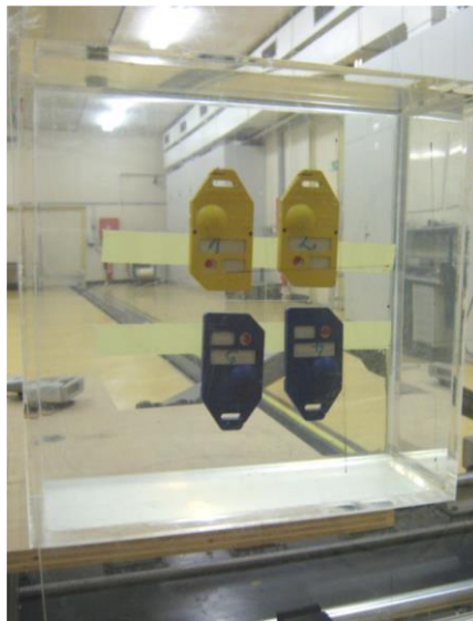
Figure 9.10 - Four whole-body dosimeters positioned on the front surface of the ISO water slab phantom (H. Stadtmann 2014).
