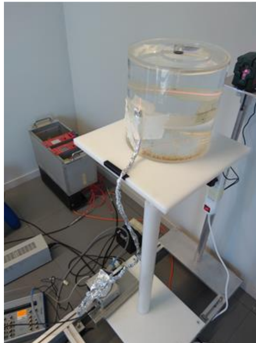
Figure 9.13 - Experimental setup for irradiating the eye lens dosimeter prototype. The dosimetric unit is placed on the surface of the water filled cylindrical head phantom according the calibration procedure (paragraph 9.3): 2.5 m distant from the tube focus (90 V bias, 1.5 V or ~ 22 keV threshold).
