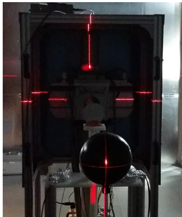
Figure 3.9 - Self-levelling red cross line laser used to align some devices to the X-ray field centre.
