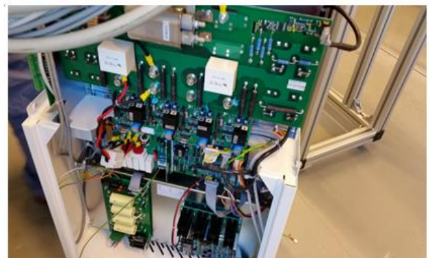
Figure 3.1 - Work in progress in the irradiation room: assembling and setting up the X-ray irradiation unit.
