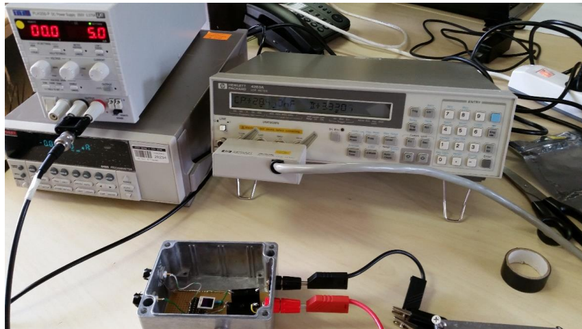
Figure 3.28 - Experimental setup of the electrical testing workstation. Voltage generator, Keithley model 6485 picoammeter, Hewlett-Packard 4263A LCR meter and metal box for the assembly of the dut.
