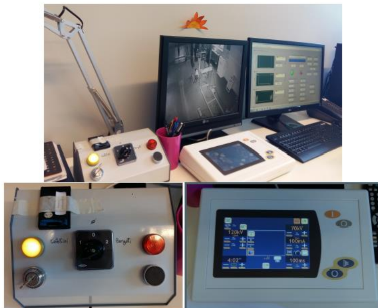
Figure 3.3 - Photograph of the control room (on the top), control console (bottom right) and device for the X-ray tube ignition (bottom left). On the latter, it has been placed a passive dosimeter for the necessary radioprotection tests.
