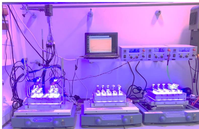
Figure III.25 In-house developed parallel photoreactors.
