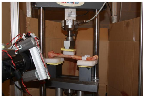
Fig. 1 Servo-hydraulic testing machine EM2/20 MicroTest, with the U10M/25-kN loading cell and two supports to create a three-point bending, from UPC
