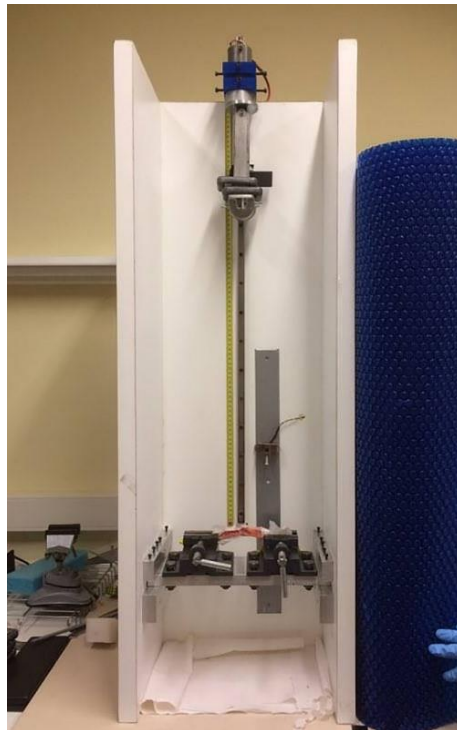
Figure 5: Drop test machine to fracture rib samples at high-speed.
