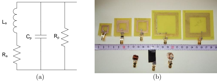
Figure 2.13. (a) Antenna circuit model for a loop antenna, (b) antennas with different sizes and number of turns.
