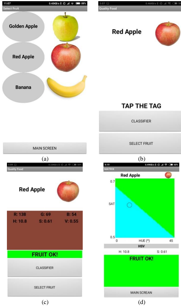
Figure 6.14. Phone screen of the developed application. (a) Fruit selection, (b) screen indicating to tap the tag, (c) representation of the detected colour, (d) decision boundaries of the training.
