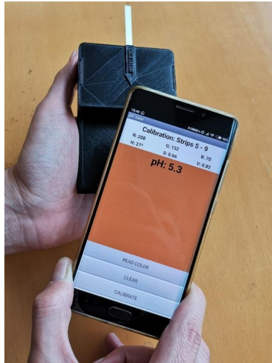
Figure 5.11. Reading the colour of a strip and calculating the pH with the Android application.
