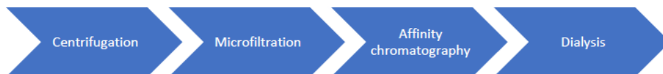
Figure 3.6. Scheme of the downstream process implemented for small scale purification of Trastuzumab.
