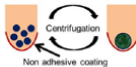
Figure 8.11. Schematic depiction of ULA+centrifugation method for 3D culture generation. Obtained from (Gupta et al., 2016).
