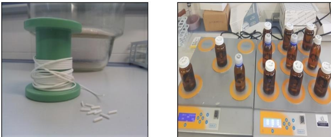
Figure 3.4. PDMS rod and experimental set-up for the rod-based extraction process.
