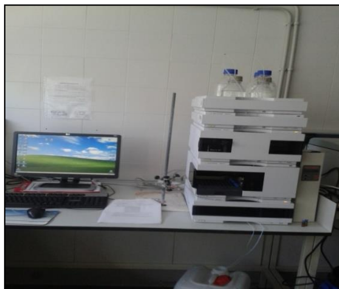
Figure 3.2. HPLC-DAD system used in the chromatographic analysis of PPCPs.
