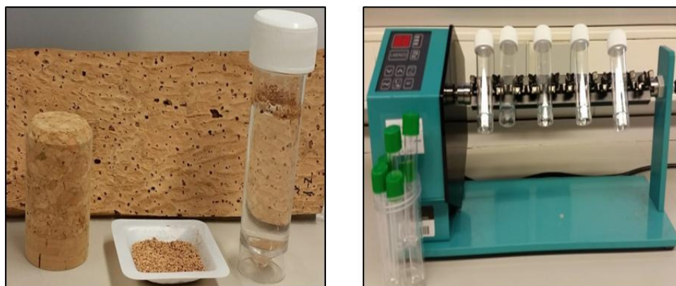
Figure 3.6. a) Granular cork and cork stopper and plate, b) experimental set-up for batch desorption experiments.
