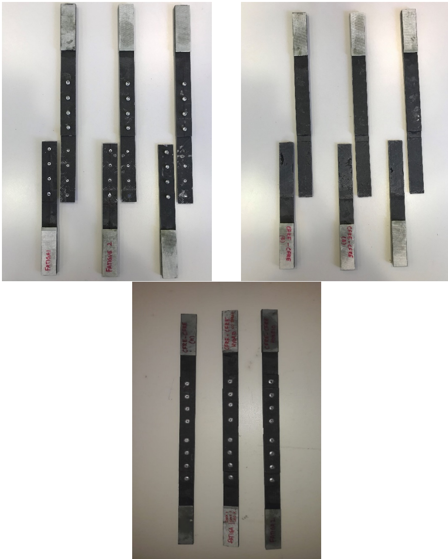
Figure 3.12: Fatigue failure of composite-composite riveted (top-left), adhesive bonded (top-right) and hybrid joints (bottom).
