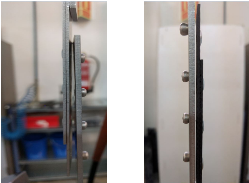
Figure 3.3: Rivet shear failure of metal-metal (left) and metal-composite (right) riveted joints [70].
