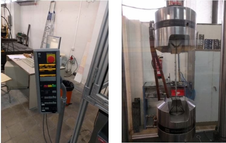
Figure 2.6: Static test machine with personal computer (left) and with loaded joint (right)
