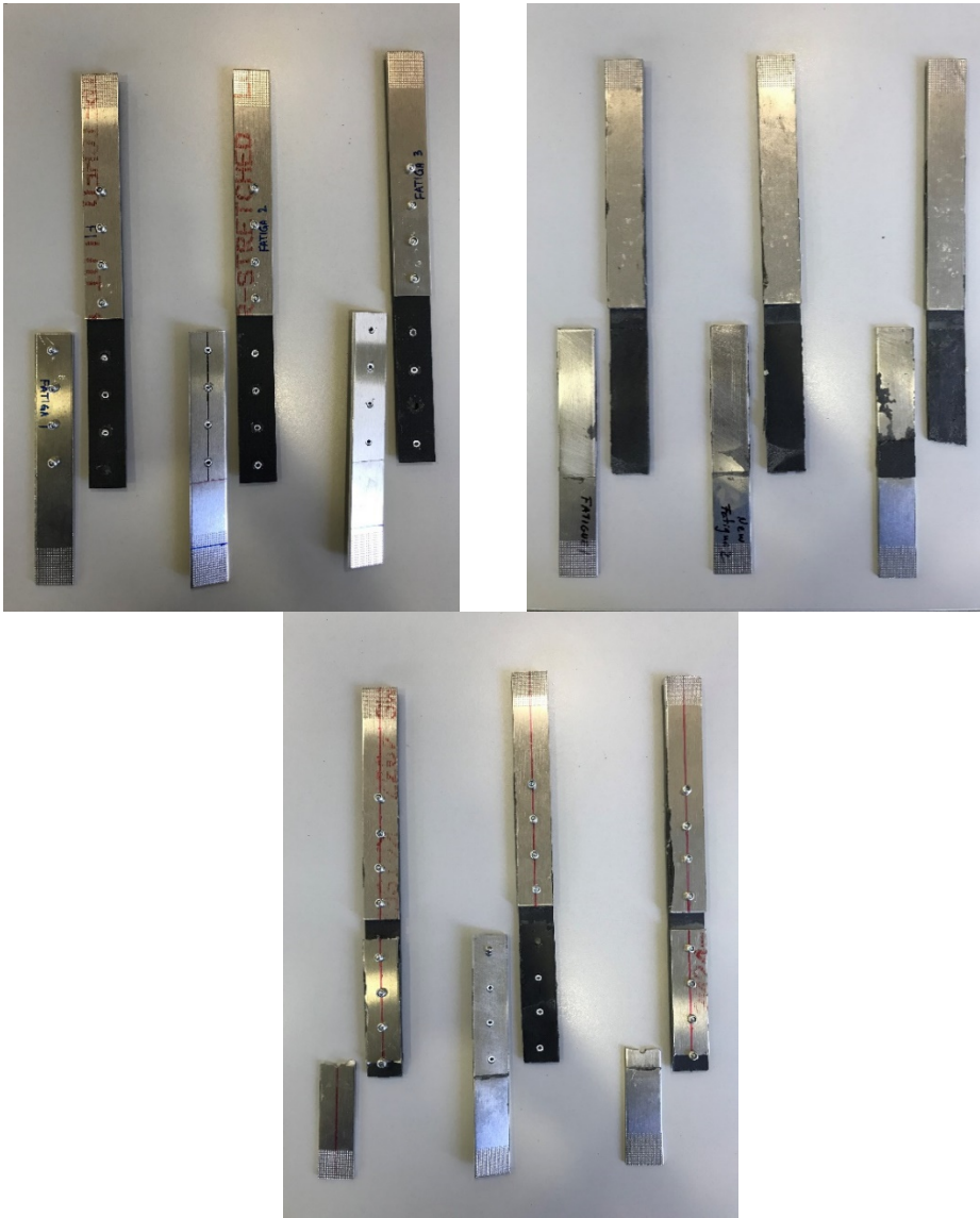
Figure 3.7: Fatigue failure of metal-composite riveted (top-left), adhesive bonded (top-right) and hybrid joints (bottom).
