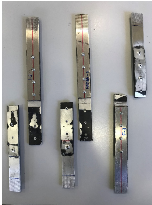
Figure 3.6: Fatigue failure of metal-metal riveted (top-left), adhesive bonded (top-right) and hybrid joints (bottom).
