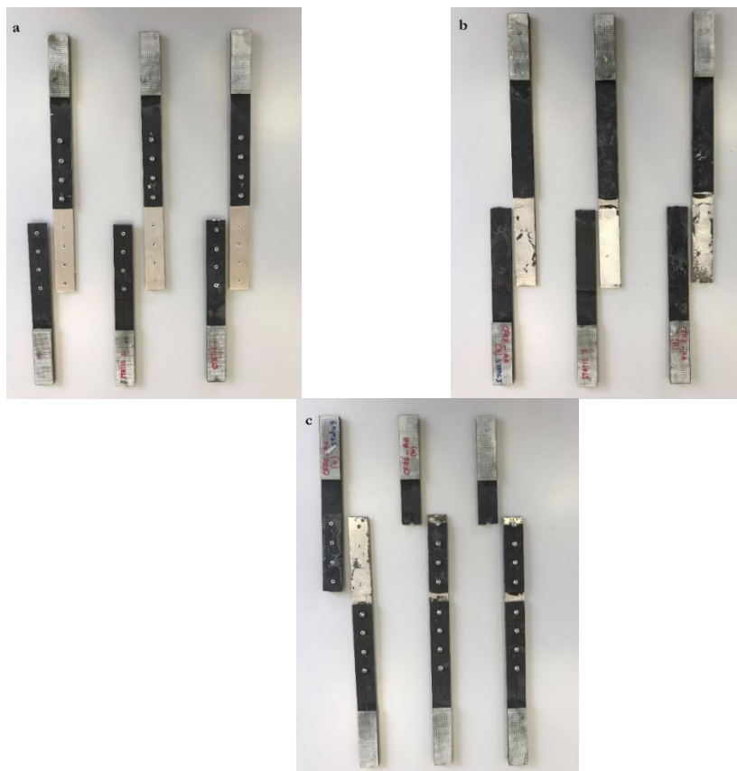
Figure 3.11: Failure of composite-metal specimens of (a) riveted, (b) adhesive bonded, and (c) hybrid joints.
