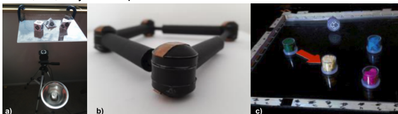
Figure 4. Interactive systems for children with VI learning. a) Low-cost tangible system for spatial awareness and tactual shape perception learning. Figure extracted from [70]. b) Accessory, 3d printed object for geometry learning. Figure extracted from [73]. c)
