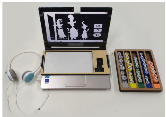
Figure 1. iCETA: headphones, computer, mirror in the camera, tangible blocks and working area on top of the keyboard.
