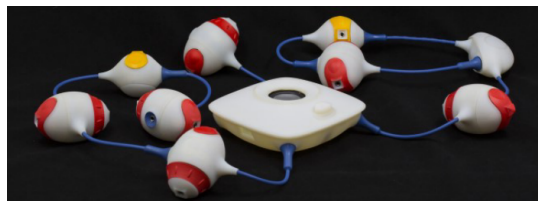
Figure 3. Torino: Different instruction beads connected to the main hub in order to create an audio-based computer program. Figure extracted from [88].
