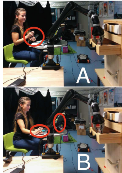
Fig. 1. The experimental setup with the Kinova Jaco arm. The participant moves the arm using (A) the joystick and (B) the graphical interface on the laptop.
