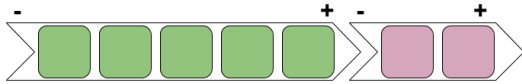
Figure 8. The block's shape constraints the way that it can be joined ensuring that magnets will not repel.
