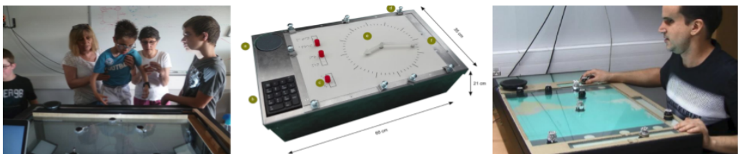
Figure 2. Left: Pupils interacting with the map of France using the Tangible Reels system. Middle: The tangible box setup. Right: A blind user zooming a map with a slider using BotMap. Figures extracted from [39].
