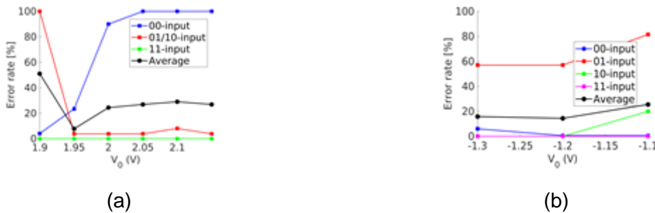
Fig. 5-18. Simulation results for error rate while considering CMOS mismatch for (a) MAGIC NOR2 and (b) CNIMP NOR2. 500 operations were realized in each case, with circuit parameters as described in Fig. 5-16c and Fig. 5-17b, respectively.
