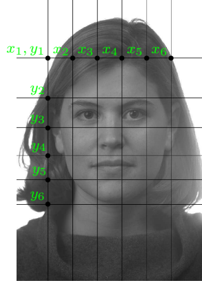
Figure 3.1: Grid based on the eye coordinates, created from the Equations 3.1 to 3.12, used to locate the face parts in the image (the points calculated with the equations are marked in green).
