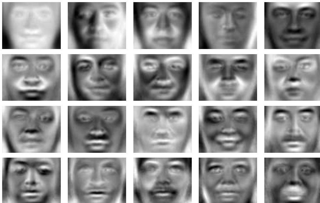
Figure 2.8: The first 20 eigenfaces , that is, the first 20 eigenvectors showed as images. The PCA was calculated with images from FERET database.
