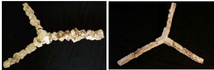
Image. [79, 80]. Left, the twisted box topology module connected parts of greensulate, right, the irregular prism topology module connected parts made of greensulate. [70]*.
