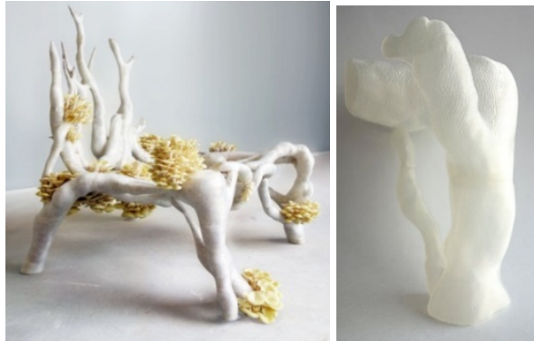
Image [13, 14]. left. The 1:1 chair mockup with the complete growth of mushroom. Right, 3D-printed segment of bioplastic shell.
