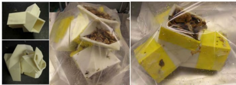
Image. [74]. left to right, the 3D container model of the irregular prism and irregular twisted box, to be filled with the greensulate material seeds. Image. [75, 76]. Left, the central connection part of the irregular prism. Right, the central connection part of irregular twisted box (the joints).
