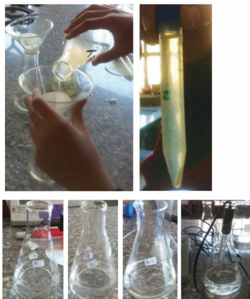
Image. [99]. Filtration of different tested fungal strains by Whatman paper (left) or centrifugation for unicellular Saccharomyces cerevisiae (right). Image. [100]. From left to right; solution (A), solution (B), the acetate buffer solution (A+B), adjusting pH of the acetate puffer solution to pH4.7 by pH meter. By author.
