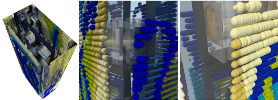
Image. [115]. Details of the self-sufficient cluster, showing from left to right, planner perspective of the lighting unite showing overlapping and conjunction between different patterns applied on four faces of the glass container, two different sides detailes shows pattern’s particles (silicon rubber) relation with transparent glass container and inner MFCs with fungus. By author.
