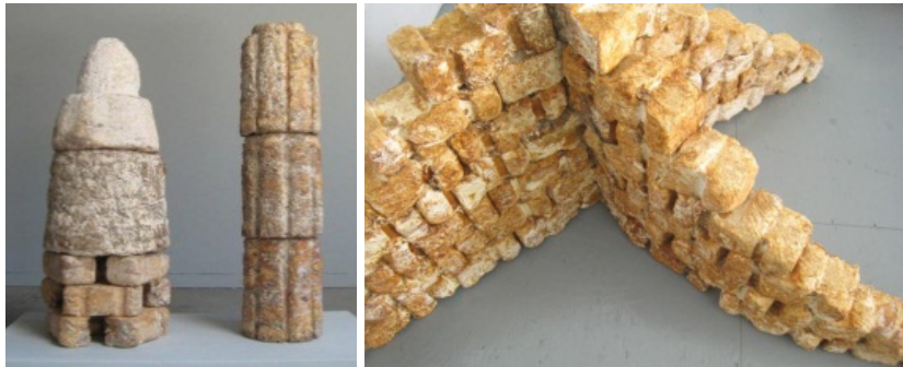
Image [9, 10]. Different assemblies of the mushroom blocks for various structural forms potentials.
