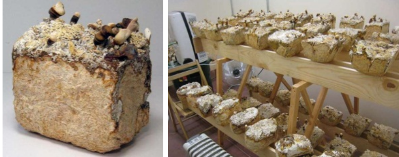
Image [7, 8]. Left, the single block made of the living mushroom mycelium and right, prototype blocks.
