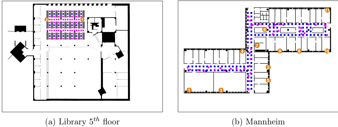
Figure 4.4: Environments for analyses of reference point selection. Blue and magenta squares represent training and test reference points, respectively. Known AP positions are identified by numbered orange circles.
