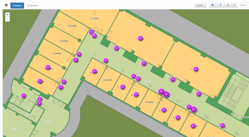
Figure 4.3: Web tool for samples visualization. The point clustering changes with the zoom dynamically.
