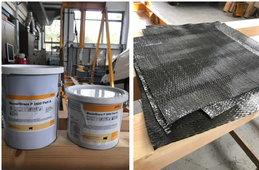
Figure 4. 34: The selected epoxy and carbon fiber textile for reinforcement
