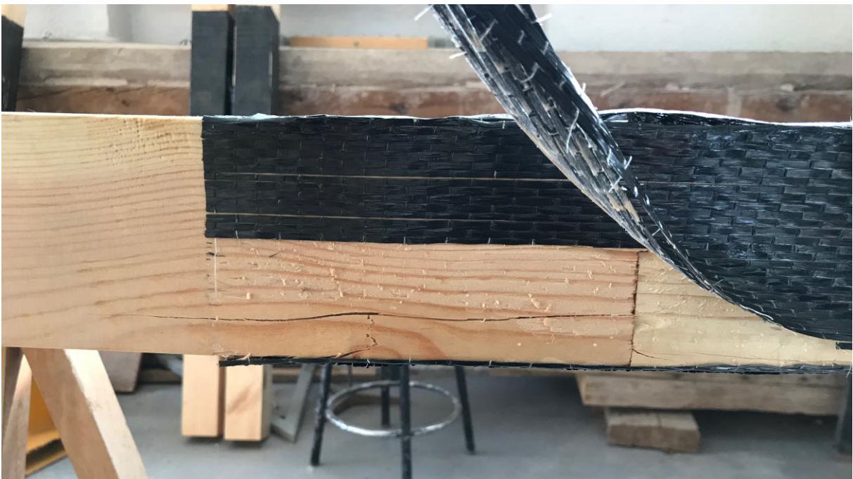
Figure 4. 48: Shear failure in second reinforced specimen (LPC1800BR) under cyclic loading
