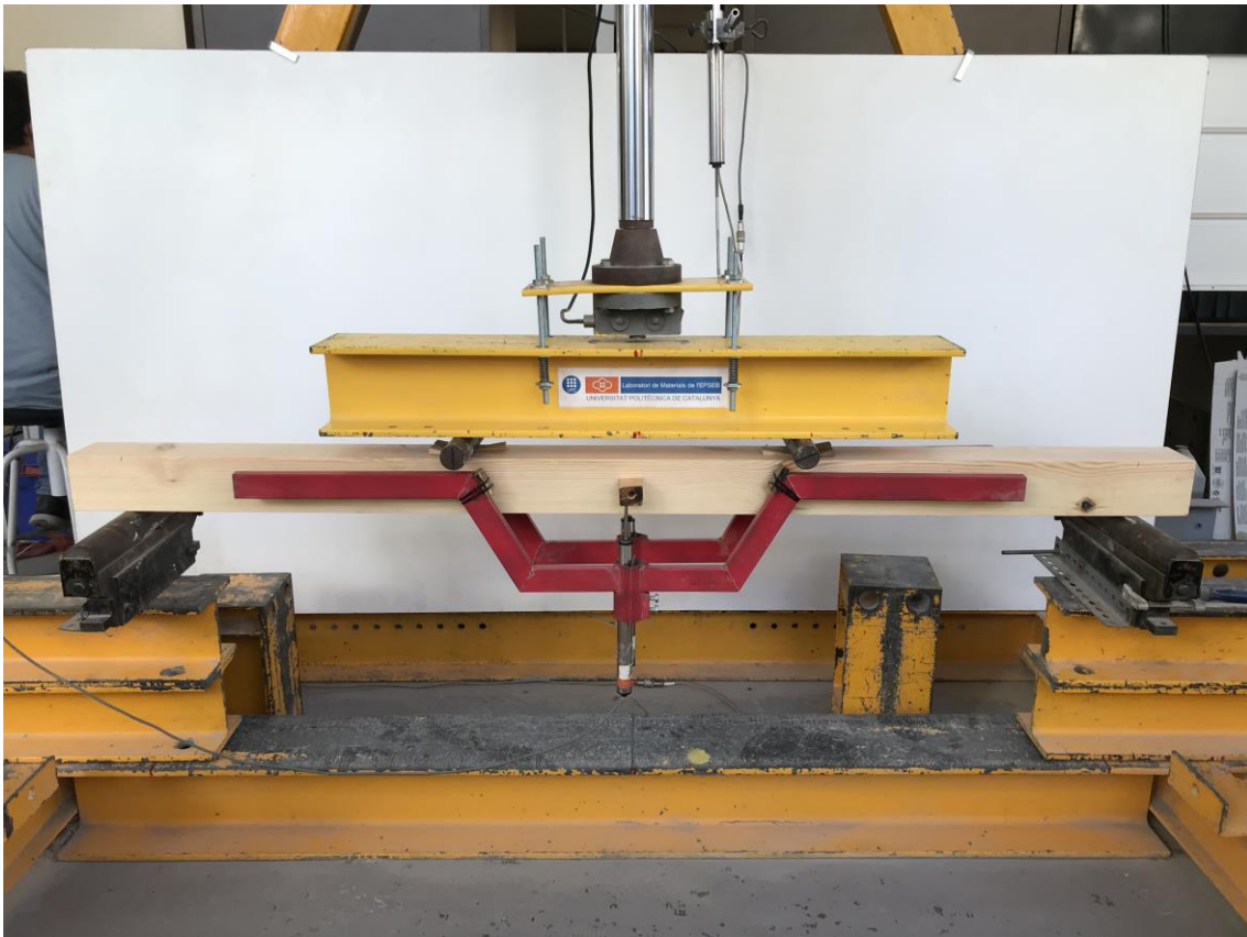
Figure 4. 17: The test set up for measuring local modulus of elasticity in bending
