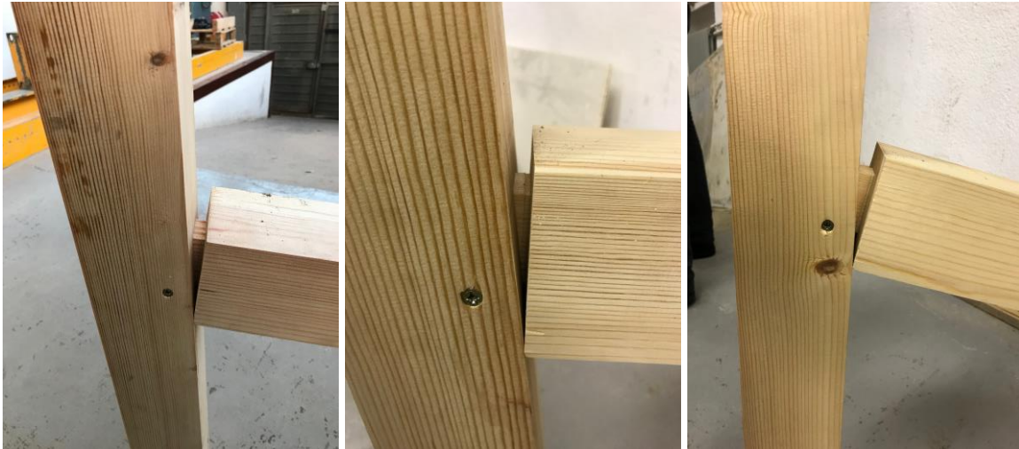
Figure 4. 57: The failure pattern of three specimens under monotonic loading
