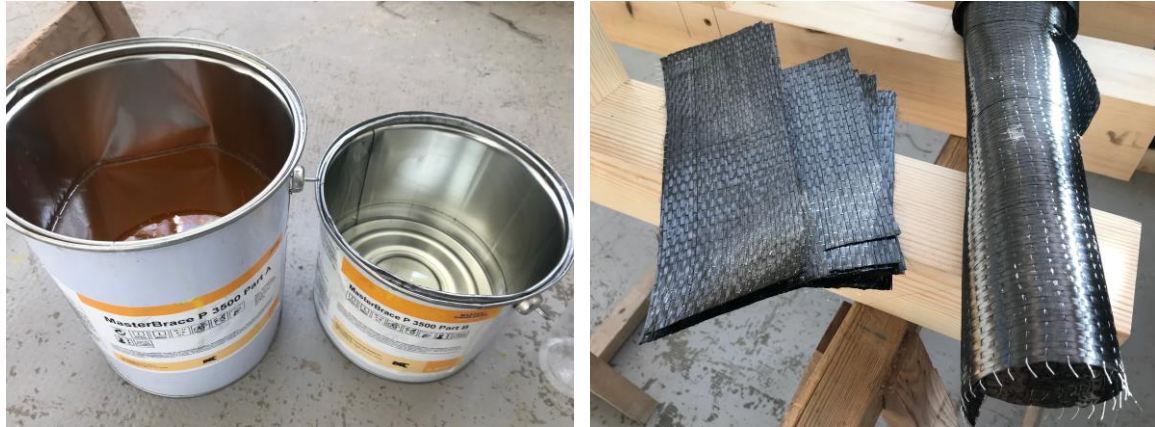
Figure 4. 60: The selected epoxy and carbon fiber textile for reinforcement
