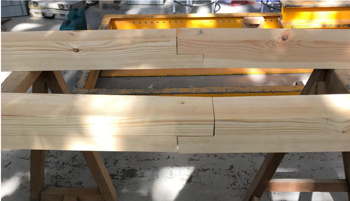
Figure 4. 32: The failure pattern of two specimens under monotonic loading
