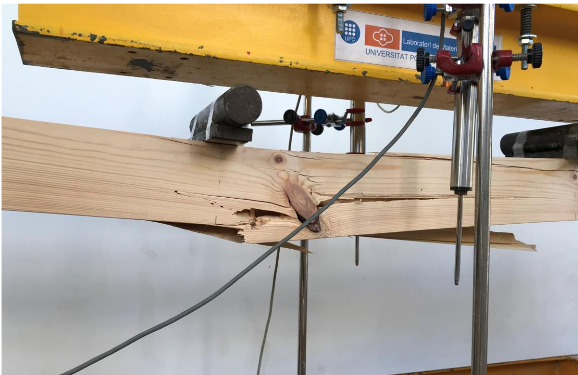
Figure 4. 25: The failure pattern of second specimen under bending due to the influence of having knot
