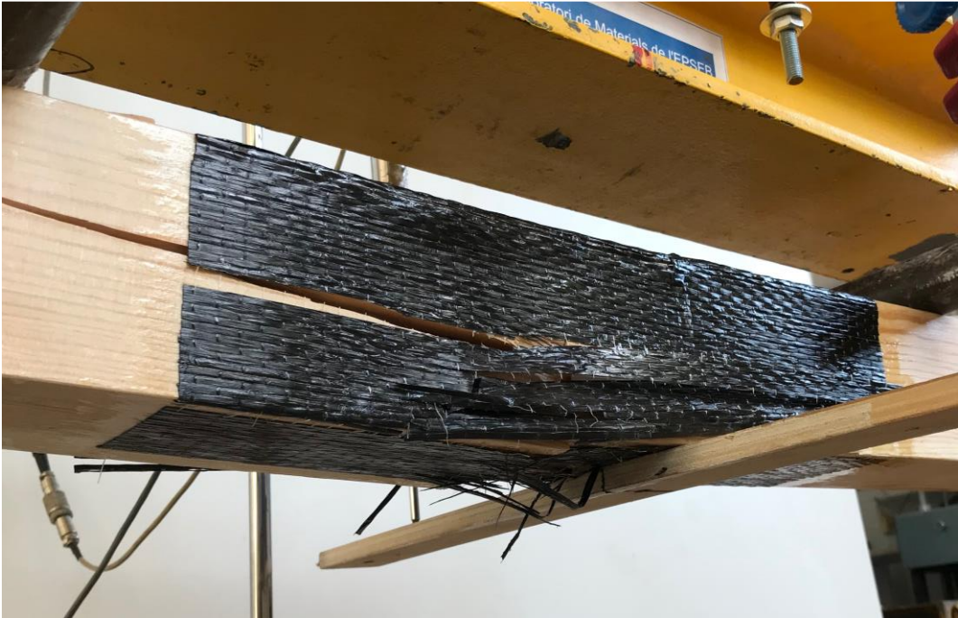
Figure 4. 38: Failure pattern of reinforced specimen (LJM1800AR) under monotonic loading
