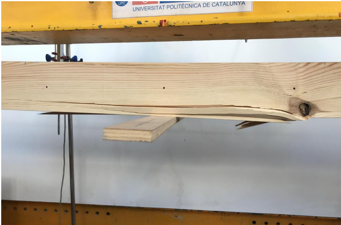
Figure 4. 26: The failure pattern of third specimen under bending
