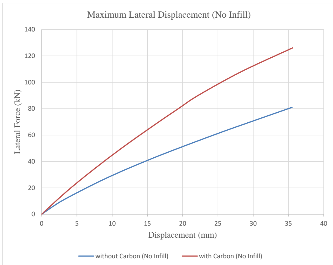
Figure 6. 26: The comprasion of global analysis results between unreinforced and reinforced frames without infill material
