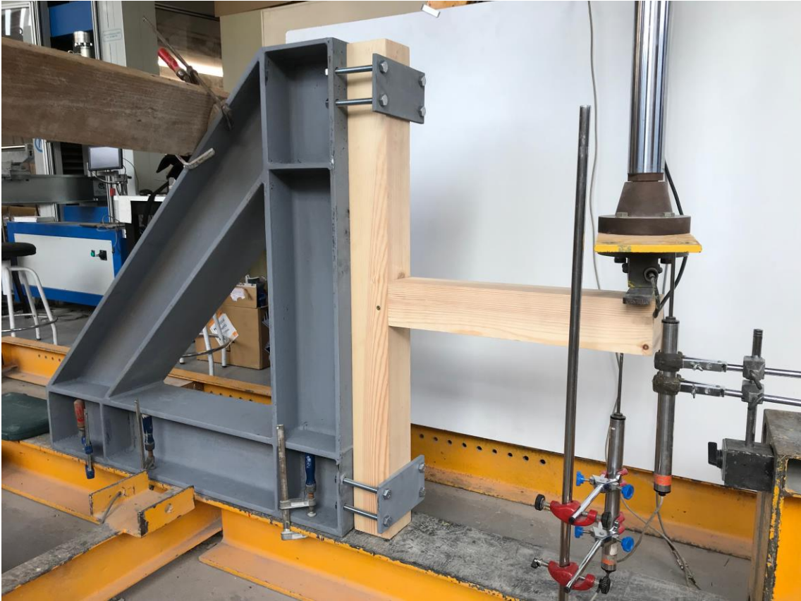
Figure 4. 65: The set up for cyclic test on unreinforced specimens
