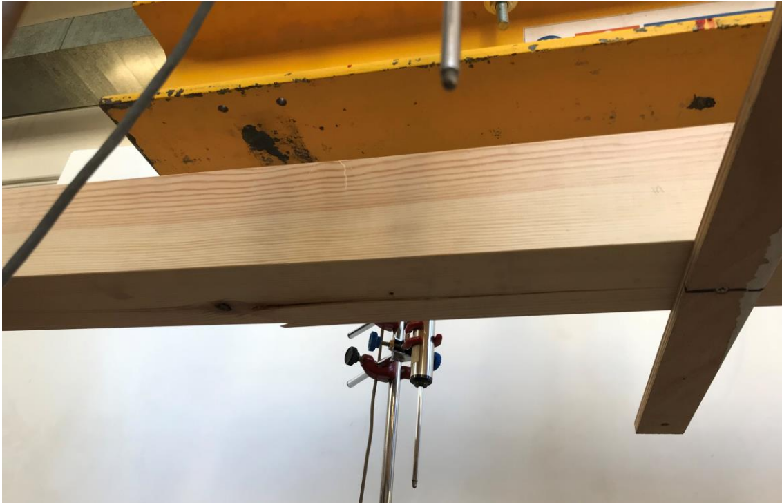
Figure 4. 24: The failure pattern of first specimen under bending
