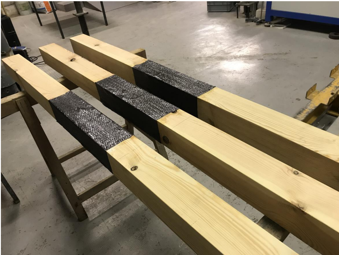
Figure 4. 35: General view of reinforced specimens for monotonic test
