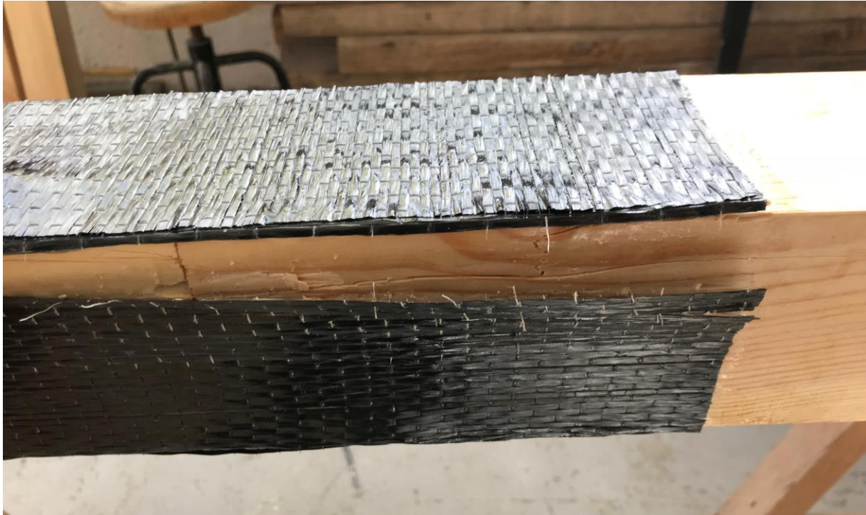
Figure 4. 49: Shear failure of third reinforced specimen (LPC1800CR) under cyclic loading
