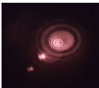
Figure 1.15: Interference pattern formed from the reflection of the top reference beam on the imaging objective. Below the biggest patterns, on the left, we can observe the reflection from the bottom viewport. On top of this reflection and also below we can observe the same interference pattern repeated. This secondary reflections come from the back reflection of the wedged window that we use in the addressing set-up.
