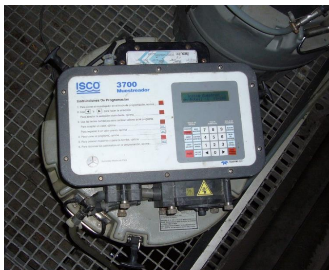
Figure 2.1: ISCO ® 3700 sampler in the WWTP-1 inflow wastewater sampling point.
