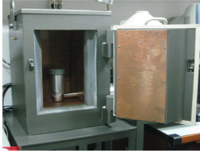
Figure 2.5: HPGe detector model GX4020 with the shielding door open ready to introduce a sample for a gamma-spectra obtention.
