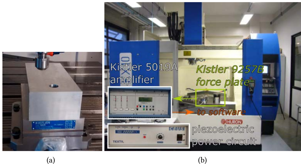
Figure 4.19. Experimental setup. a. Detail of workpiece attached to a Kistler dynamometer. b. HURON KX10 milling machine where experiments were developed.
