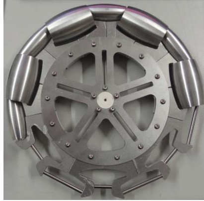
Fig. 1.6. Image of the internal structure of one of the omnidirectional wheels used in the APR robot.
