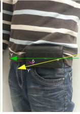
(c) Smartphone in the nonexpected position and orientation on the waist. There is an angle of error in the transverse body plane between the device's real (green arrow) and expected (yellow arrow) orientation.
