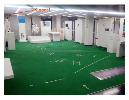
**Figure 6.5:** The experiment venue. Markers on the floor indicate start and end points and numbered reference points for standing in a predefined orientation. Additional markers also show which part of the area is covered by which Kinect device.
