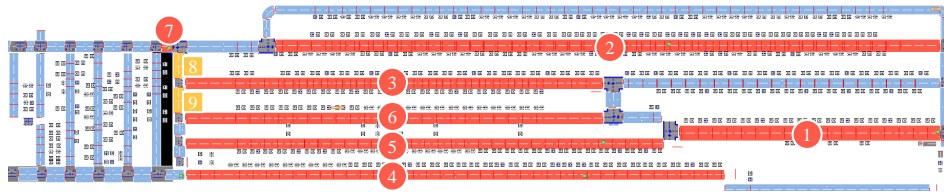
Figure 6.7: A heat map based on the workshop’s layout and the number of interferences computed through the simulation of the scenarios A and B. Notice that the level of interferences is quite similar in both scenarios. However, those scenarios’ interferences are not the same ones, as observed in table 6.6.
