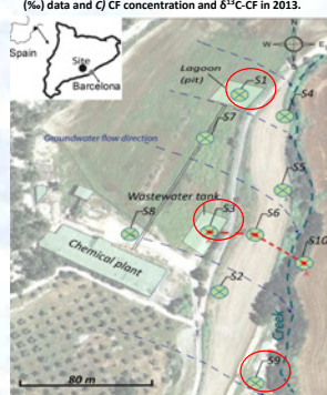
✓ From 2006 to 2013, redox conditions in S1 have evolved from iron reducing to more oxidizing, whereas S3 and S9 maintain increasing reducing conditions in depth (from oxalic to anoxic). In S3, δ 34 S- 32 S 0 (‰) enrichment in depth might indicate sulfate-reducing conditions .
