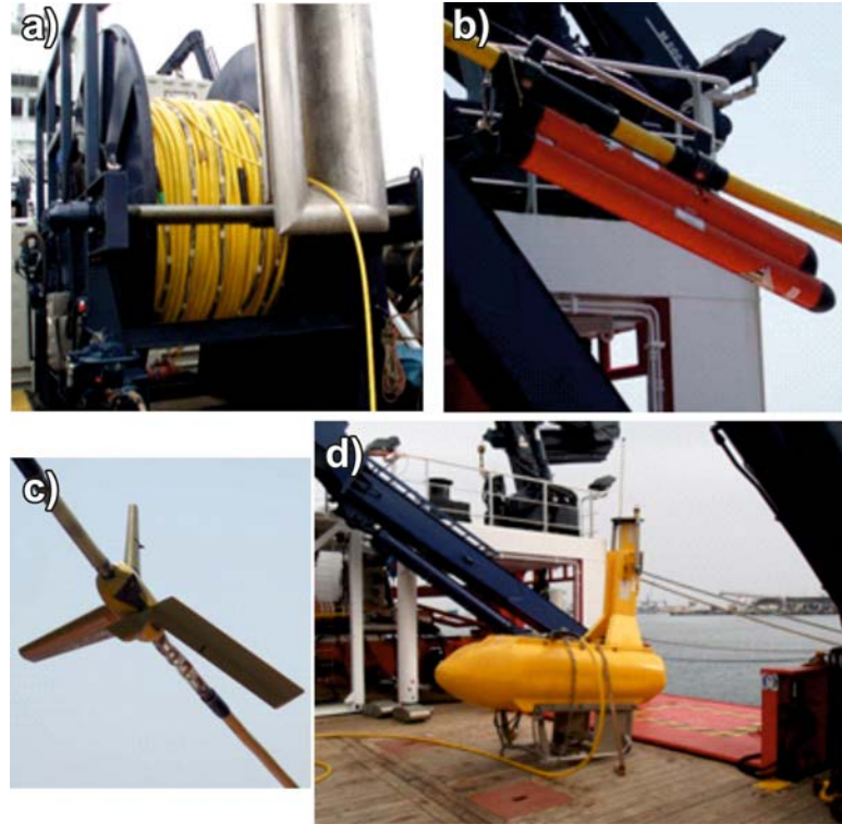
Figure 2.16: Elements of a MCS experiment, from Gómez de la Peña, 2017. (a). Streamer composed by the hydrophones. (b) Compass. (c) Bird. (d) Tail buoy.
