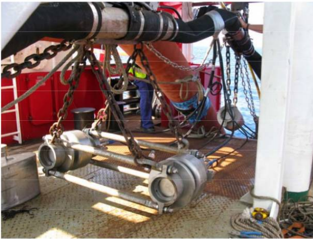
Figure 2.8: Active seismic sources. (a) Seismic source showing an air gun cluster of the gun array installed on the starboard side of the RV Sarmiento de Gamboa during the TOPOMED (2011) cruise (from TOPOMED-GASSIS report, 2011). (b) Vibroseis truck. For generating the seismic source, the truck hits the floor at a certain frequency (Dean, T. et al., 2013).
