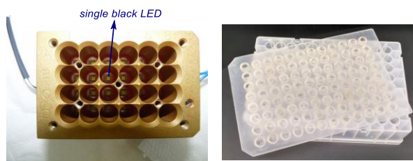
Figure 2.31. Left: 24-well aluminium block fitted with 24 single black LEDs on the bottom. Right: 96-well LC block with a silicon-rubber storage mat.
