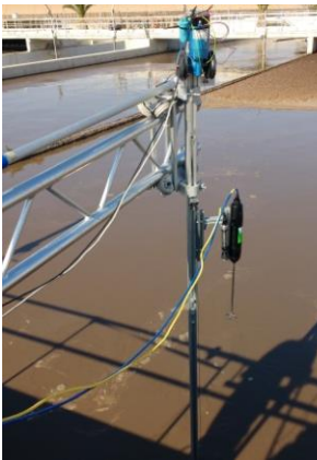
Figure 3.21. Laboratory probe (left) and field probe (right) of the Vectrino Nortek measuring in full-scale tanks and the scheme of functioning.
