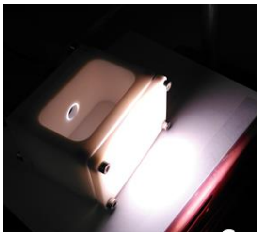
Figure S7. Photoelectrochemical cell used in this work.
