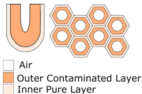
Figure 2.3: Illustration of the pure inner and contaminated outer layer of aluminium oxide formed during the anodization process.
