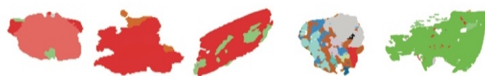
Figure 4.33. False color images showing the minerals association of CGM for the Penouta ore (a, open pit; b, tailings).
