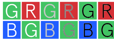
Figure 6.4-3 Final colors after demosaicing, with the pixels of the edge in a grayscale
