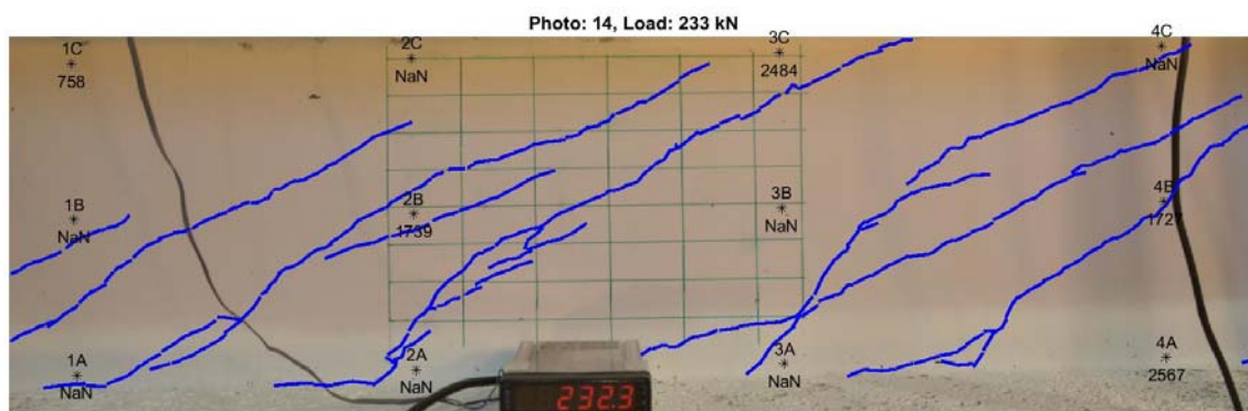
Figure 5.3-22 Deformation of the strain gauges. Test I124 Rect [ \mu\text{m}/\text{m} ]
