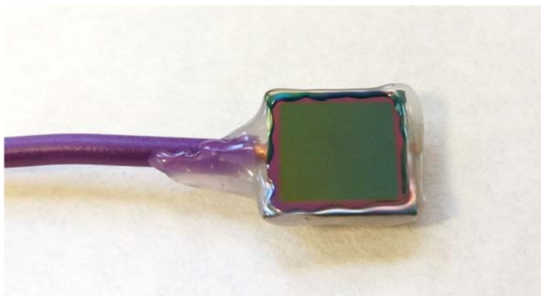
Figure S1. Picture of a n + p-Si photoanode presenting the 1.2 x 1.2 cm 2 Si chip with an active area of 1 x 1 cm 2 , defined by a perimeter of 100 nm of SiO 2 thick insulator layer. The Si chip was protected by TiO 2 -ALD and Ag paint soldered to a Cu wire, and further encapsulated with epoxy resin.
