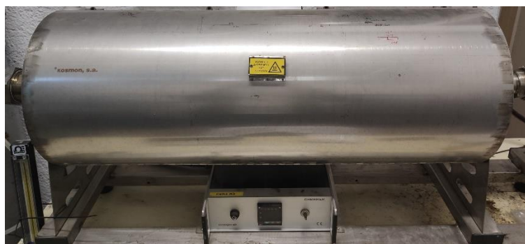
Figure 36. Purpose-made tubular furnace used for the carbonization.
