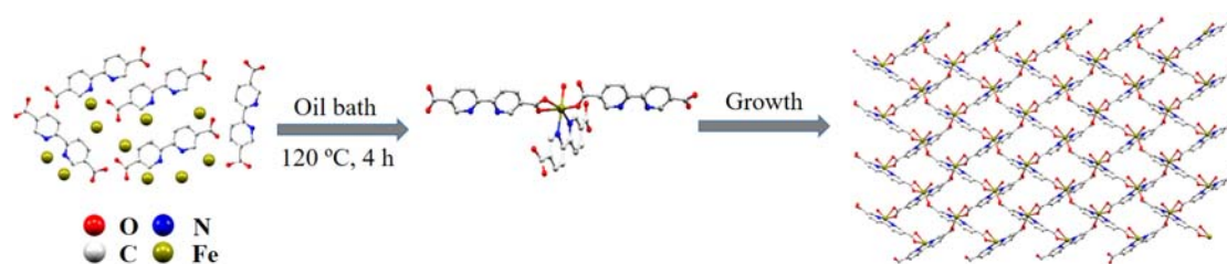
Figure 38. Schematic illustration of the synthesis and crystal growth of Fe-bpydc.
