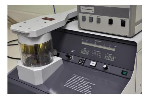
Figure 3.9 Photograph of sputter coater used for sample preparation prior to SEM.
