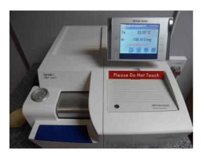
Figure 3.14 Photograph of thermogravimetric equipment used for thermal degradation analysis.
