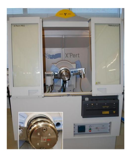
Figure 3.11 Photograph of X-ray diffraction equipment.
