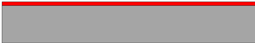
a) Sacrificial layer deposition.
