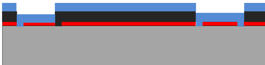
d) Metal 1 deposition.
