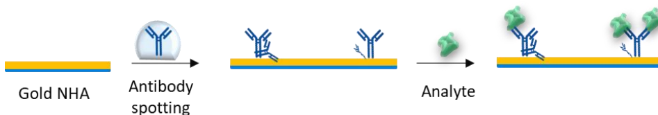
Figure 4.7: Schematic representation of the direct antibody adsorption protocol.
