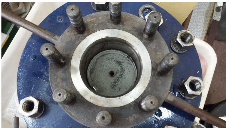
Figure 51. Fly ash inside the sample chamber.
