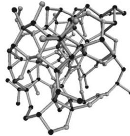
Figure 1.10 Typical structure of amorphous carbon [McCulloch DG, 2000]
