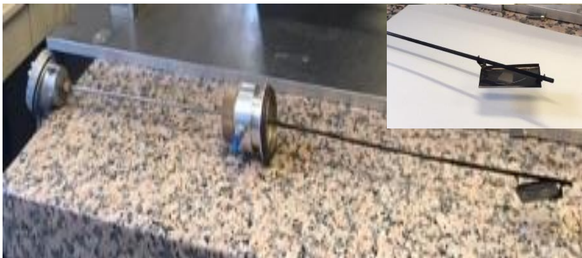
Figure 4.9 Vacuum feedthrough with linear movement, stainless steel blind, 3mm Ø, k-type thermocouple-arm and molybdenum holder (right end)
