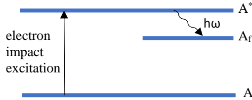
Figure 3.17 Schematic of electron impact excitation followed by a radiative de-excitation process
