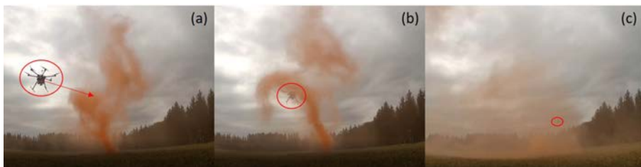
Figure 1.8: Smoke column (a) before, (b) during and (c) after a DJI M600 hexacopter flies over it (Source: Unpublished results).
