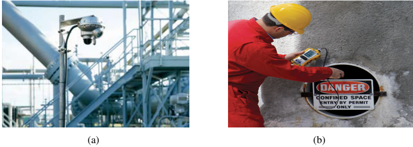
Figure 1.2: (a) Ultrasonic detector used to detect gases escaping from pressurized leaks 3 ; (b) Human operator monitoring gases in a sewer tunnel using a PID 4 .
