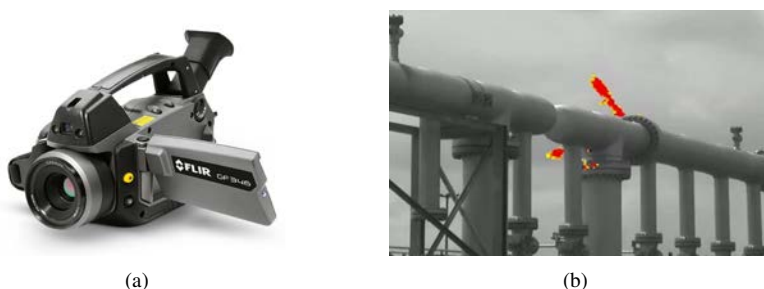
Figure 1.43: (a) OGI camera 19 (Model: GX320, FLIR Systems Inc.); (b) Visualization of a gas leak (colored in red) using an OGI camera 20 .)
