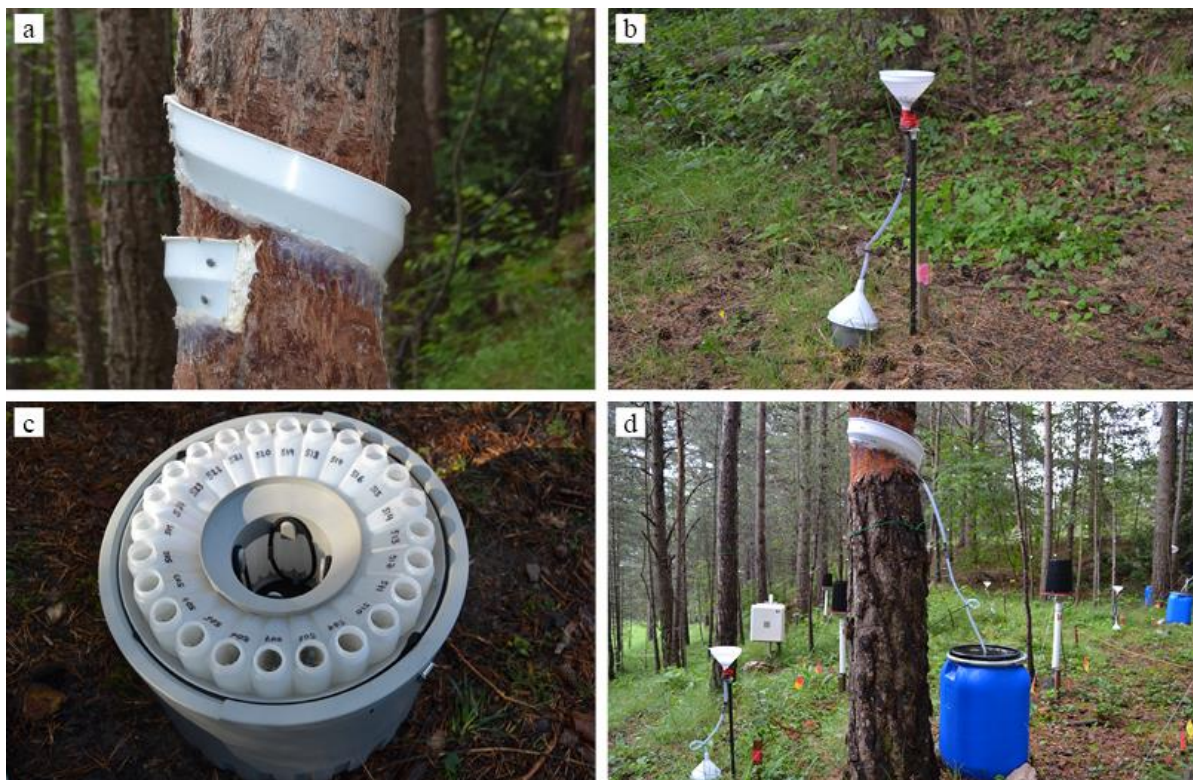
Figure 2.5. (a) Stemflow ring; (b) Throughfall collector; (c) Automatic water sampler; (d) Stemflow collector.
