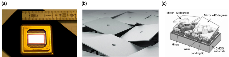
Figure 2.2: (a) Texas Instruments DLP digital micromirror device (DMD); (b) Micromirror arrangement on a DLP chip; and (c) A schematic structure of a single DMD micromirror (Extracted from [46, 50, 51]).
