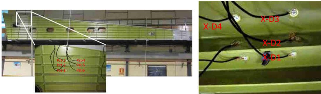
a). skin panel b.) Mass adding damage description.
