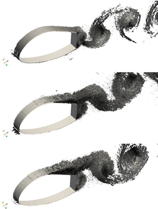
Figure 2.10: Isosurfaces of the second invariant of the velocity gradient tensor colored by the velocity magnitude on a FX77-W-500 airfoil. The flow conditions were: Re = 2.75 \times 10^6 at the AoA of 0^\circ (top figure), 12.5^\circ and 16^\circ (bottom figure).
