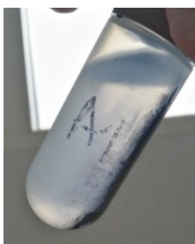
Figure 4-5-10. Complete decolourization after a centrifugation process for 10min of an Acid Black 58 solution treated during 2h with Mn-Al MPs.
