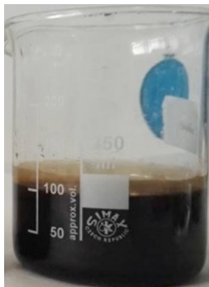
Figure 4-5-2. (Left). Coloured water with 150mg / L of Black Acid 58.
