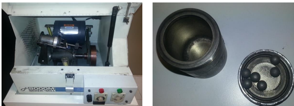
Figure 3-1-1. (a) Mechanical mill Mixer / Mill 8000M. (b) Work cylinder and mill ball (GRMT).
