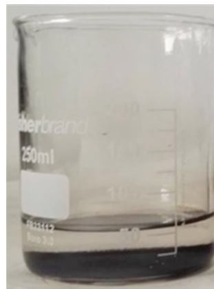
Figure 4-5-2. (Left). Coloured water with 150mg / L of Black Acid 58.
