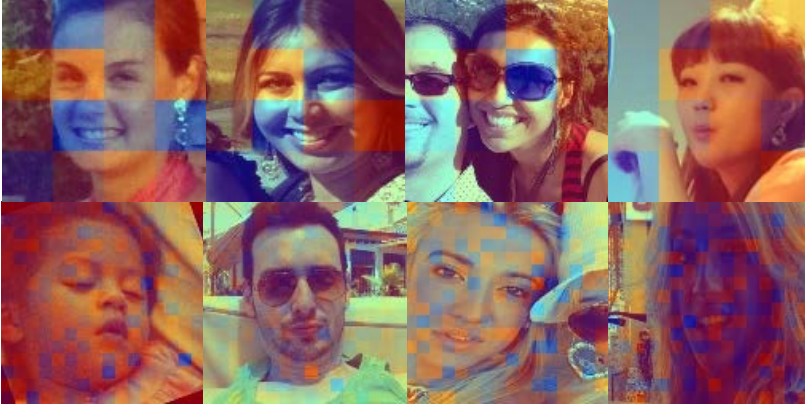
Figure 3.4: The predicted attention grid. The top row corresponds to a grid learned with k = 4, n = 4 , and the bottom row to k = 16, n = 5 . High attention is shown in red, and low attention in blue. As it can be seen, the attention grid predicts low values for background, glasses, and rings
