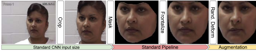
Figure 2.3: Pre-processing pipeline. The different stages of data pre-processing that were applied to the image. First, the image is aligned and cropped so as to fit the standard CNN input size. Then, it is masked and frontalized using piece-wise affine warping to match the standard pipeline proposed in [72]. Finally we perform data augmentation by applying landmark-based random deformations.
